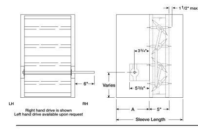
The standard location of a damper mounted in a factory sleeve ("A" dimension) is shown below. The damper can be positioned at other locations within a range of 6 in. (152 mm) to 12 in. (305mm) for the "A" dimension.
